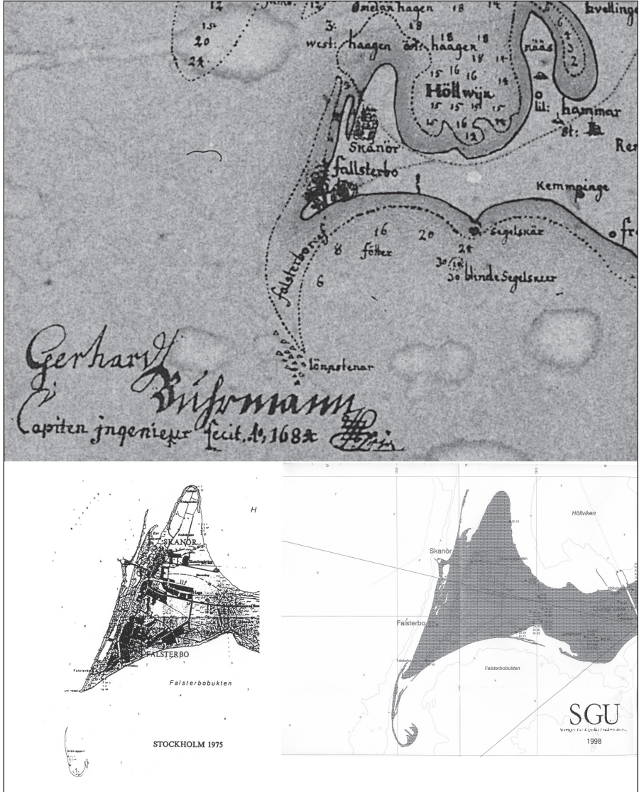
Fig. 1. Maps of the Falsterbo-Skanör peninsula dating from 1684, 1975 and 1998. The differences in the geographical survey show how the seashore has changed with time. Most clear is the shape and position of the small island, located at the tip of Falsterbo, called Måkläppen. The original map from 1684 was made by the engineer Gerhard Buhrmann and is part of the Military Archives. The maps from 1975 and 1998 belong to Sveriges Geologiska Undersökning.
