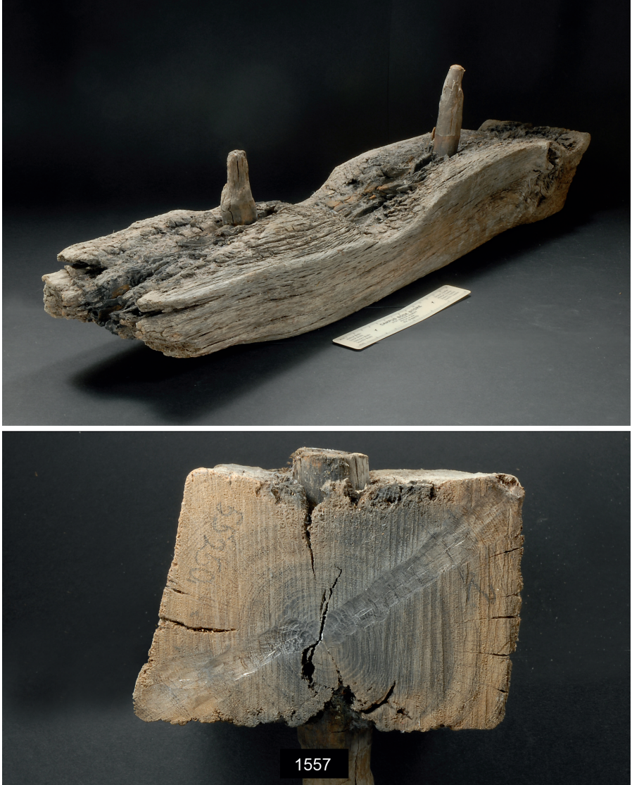
Fig. 17. Board which was part of a ship wrecked on the island of Måkläppen (Falsterbo) collected in 1990. Dendrochronologic analysis based on the pattern of the rings found in its cross section dated the board to the year 1557. Upper figure: the piece of the board which was analysed (62.0x11.6x7.3 cm) showing its two wooden plugs (length 16.0x diameter 2.5 cm). Lower figure: the cross section of the board displaying the concentric rings used in the dating.
