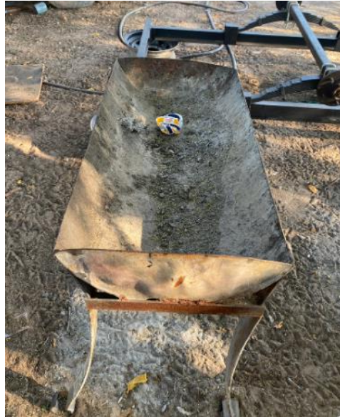
Figure 5. A metal brazier fabricated from a discarded geyser.
