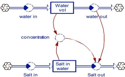
Figure 6: The combined CLD and SFD allows for us to realise the differential equation structure.
