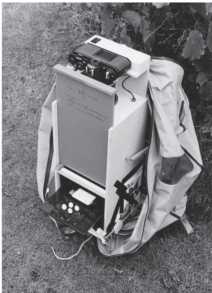
Figure 3. The apparatus in action. It is placed on ground and partly freed from the waterproof. A clutch of four Linnet Carduelis cannabina eggs are placed on the shelf, the remaining egg holes are closed with black tape, and a piece of writing tape with notes is affixed to the glass plate. The next steps are to push the shelf into the box, close the sliding door, and then photograph.
