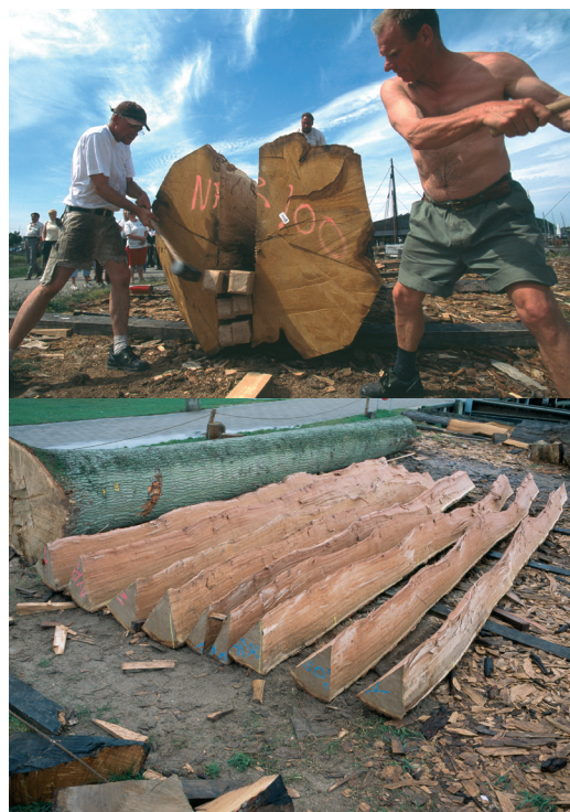
Fig. 3. Cleaving of an oak log to provide timbers for the production of radially-oriented planks. Photos by Werner Karrasch, Viking Ship Museum in Roskilde.
