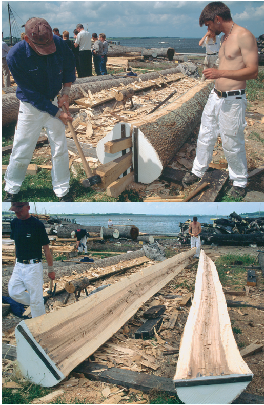
Fig. 6. Cleaving of an ash log to provide timbers for the production of tangentially-oriented planks. The outlines of the planks are marked in black on the log. Photos by Werner Karrasch, Viking Ship Museum in Roskilde.
