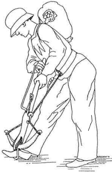
Fig. 8. A medieval soldier spanning his crossbow with a crossbow bender ( krihake ). From Ekdahl 1998, p. 142, fig. 11.12.
