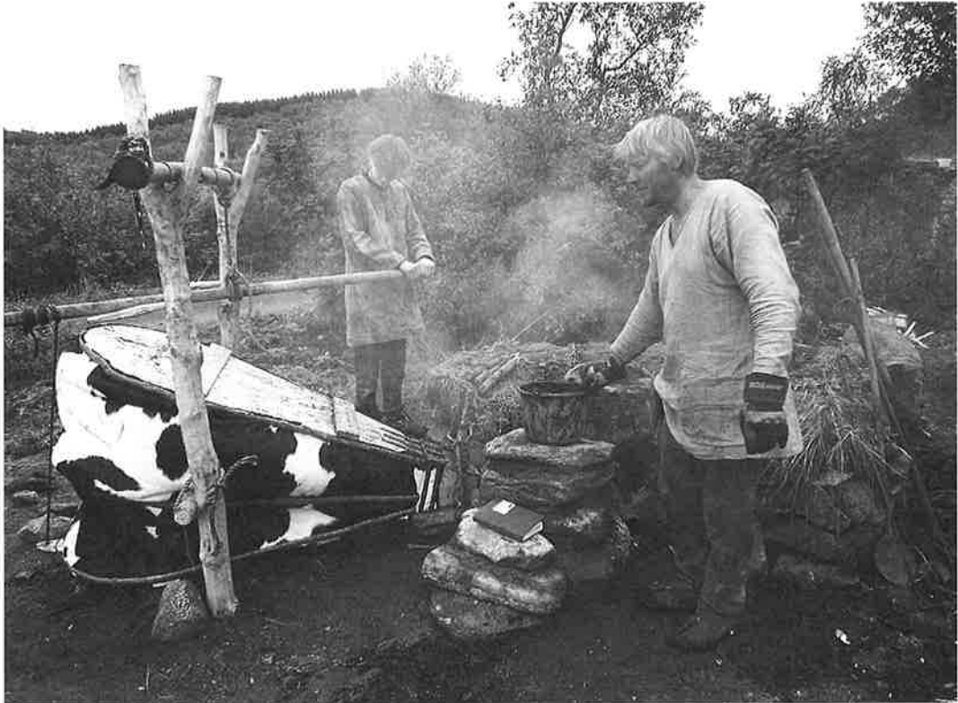
Fig. 5. Experimental smelting of bog ore in a 700 AD reconstructed slag tapping shaft furnace at Lofotr Viking Museum. The author to the right and his son to the left – action mediated knowledge. Photo Lofotr Viking Museum.
