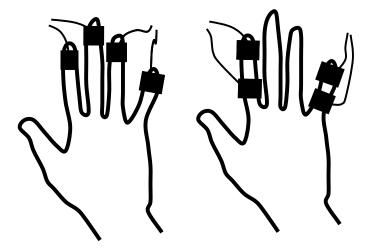
**Fig. 1: a)** One pair of electrodes attached on pads of the first and second fingers and another pair attached to the pads of the third and fourth fingers.
