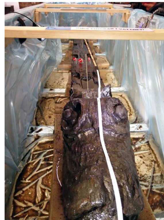
The Griffin head and the beam in the drained storage tank. The wooden pins and flags are placed in the holes where the density profiles were taken. Photo: David Gregory, Nationalmuseet
