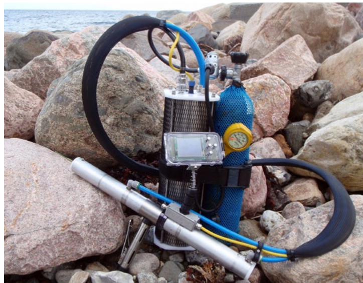
Prototype of the wood density profiler. Photo: Robert Pedersen, AKUT
