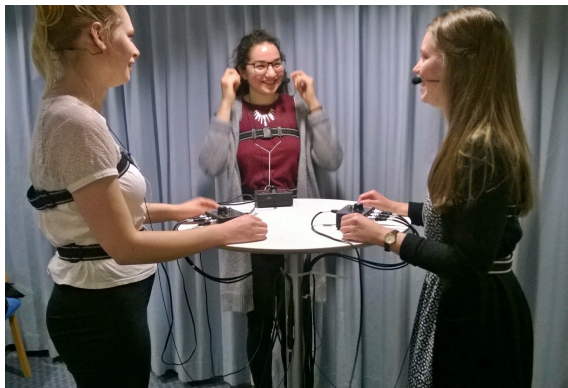
Figure 1. Students in the Phonetics Laboratory wearing transducer belts, each connected to a RespTrack, during a recording session.
